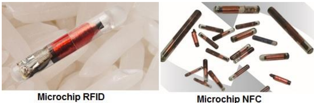
Figura 2.13 - Microchip RFID x Microchip NFC
