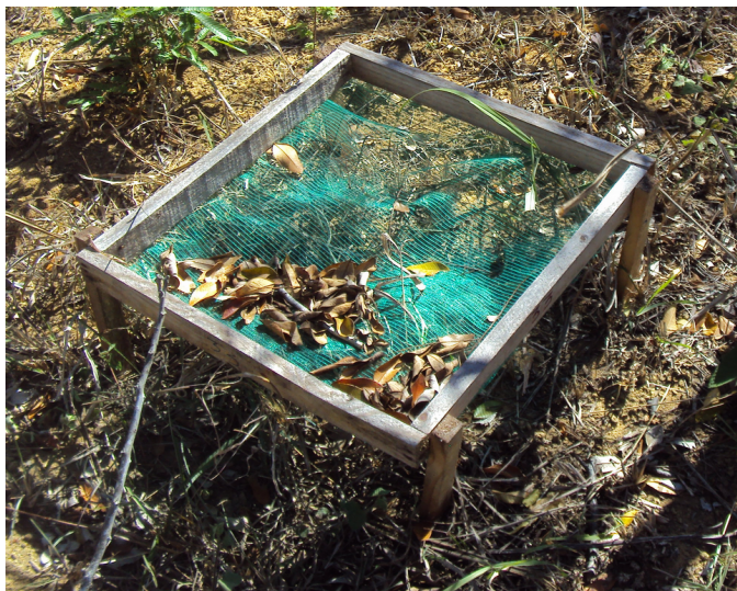
FIGURA 2: Coletor de serapilheira instalado no campo. FIGURE 2: Litter collectors installed in the field.
