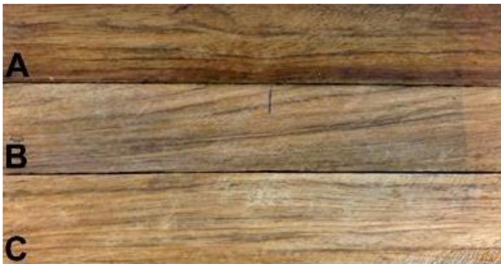
Figura 2 - Madeira de Micropholis sp. A: 200°C; B: 160°C; C: Controle. Figure 2 - Wood of Micropholis sp. A: 200°C; B: 160°C; C: Control
