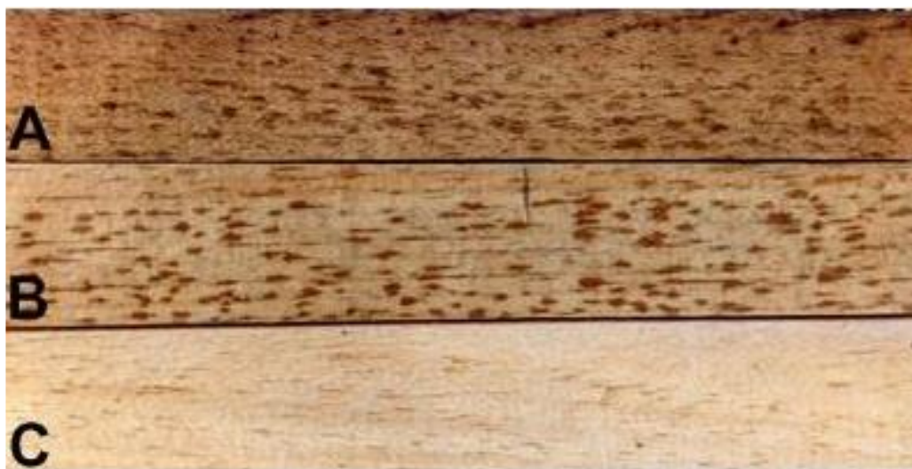
Figura 1 - Madeira de Pinus sp. A: 200°C; B: 160°C; C: Controle. Figure 1 - Wood of Pinus sp. A: 200°C; B: 160°C; C: Control.
