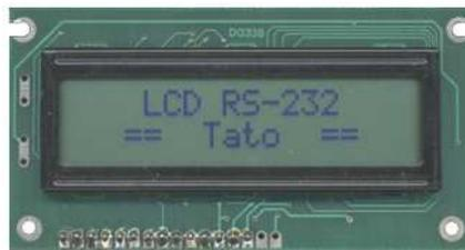
**Figura 24**-Display Serial TS-216
